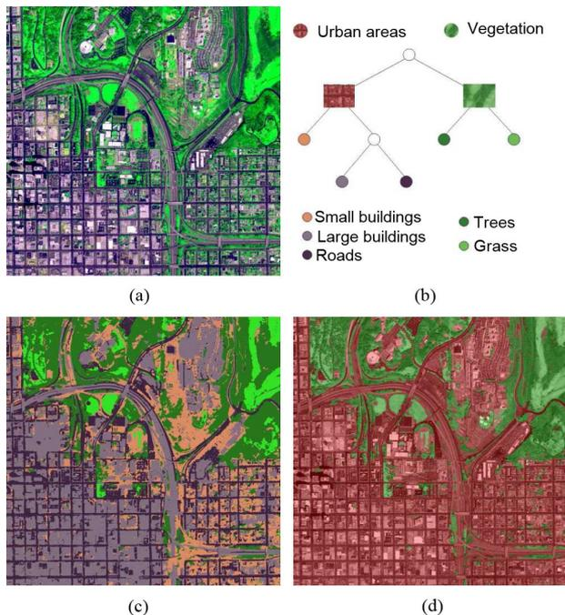
Fig. 7. IKONOS image segmentation: 4m-resolution multispectral image, size  $501 \times 501$ , false color representation of the original image (a); 5-class pruning of the retrieved tree structure (b); 5-class segmentation (c); Top-level classes: urban areas and vegetation (d).
